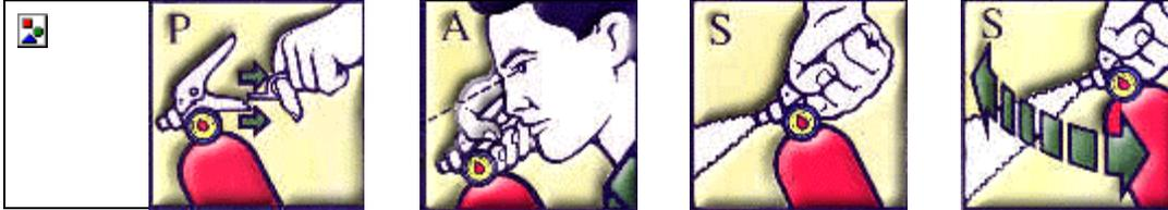
It's easy to remember how to use a fire extinguisher- simply follow the steps- "P-A-S-S" **P**ull the **P**in: Pull the pin at the top of the extinguisher that keeps the handle from being pressed. Break the plastic seal as the pin is pulled.
